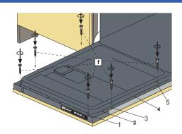
21 Attach the doors using the screws (f) provided. Ensure screws will not come through the front of the door before beginning.
