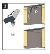
Take the supplied moisture resistant foil (a) and stick it to underside of the counter top.
