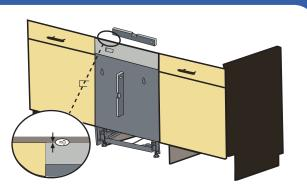
Raise and level the appliance. Level the appliance. Ensure there is no gap between the appliance and the counter top.
