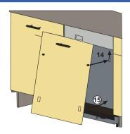
**19** Lift the door into place. Align the fitted screws (d). Push the door in and up. Push the lower half to stick the adhesive pads to the appliance.
