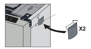
Add a supplied side spacer (c) to either side of the appliance.
