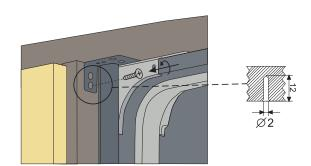
**24b** Stone or ceramic counter tops: Attach into the sides of the adjacent units, using the small screws (h) provided.
