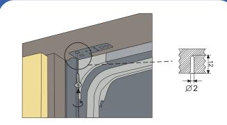
**24a** Wooden counter tops: Screw vertically up into the counter each side, using the small screws (h) provided.
