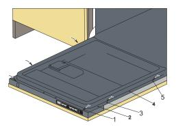
20 Fully open the door and remove the 1st, 3rd and 5th screws illustrated, from each side of the dishwasher inner.
